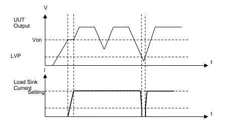
Figure 3-26 When Von Point is not set to 0V with Protection
