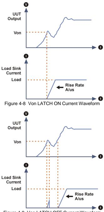
Figure 4-9 Von LATCH OFF Current Waveform
