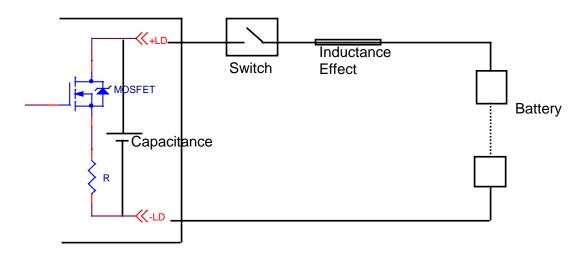
Figure A-1 Wire Connection of Electronic Load & Battery
