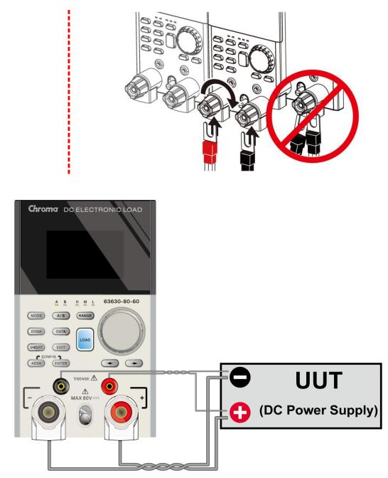
Figure 2-4 Load & Remote Sensing Connection
