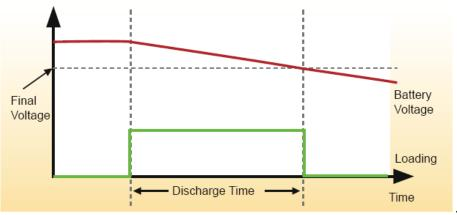
Figure 3-19 Timing Measurement Function
