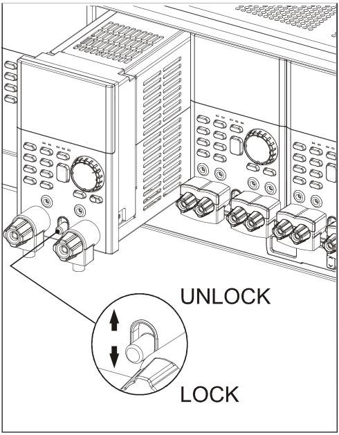
Figure 2-2 Installing Modules in the Electronic Load
