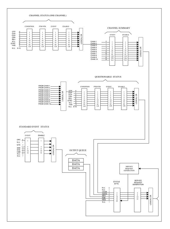
Figure 6-1 Status Registers of Electronic Load
