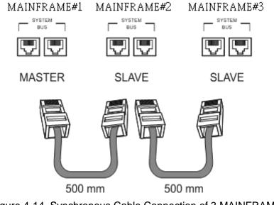
Figure 4-14 Synchronous Cable Connection of 3 MAINFRAMES
