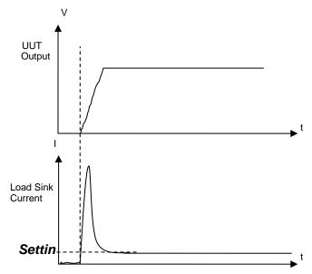
Figure 3-24 When Von Point sets to 0V without Protection
