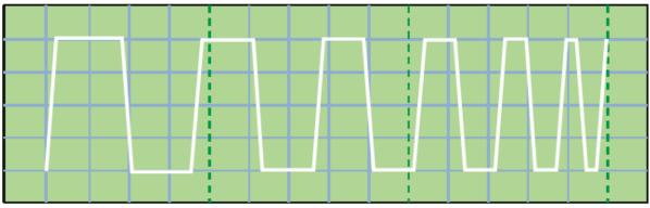
Figure 3-12 CC dynamic Frequency Sweep Current Waveform
