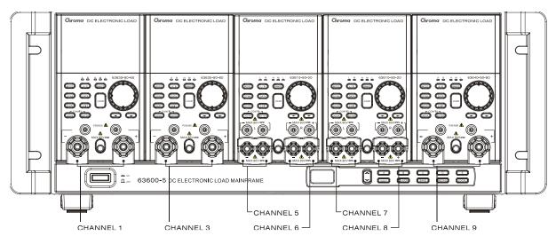
Figure 2-3 Example of Channel Number
