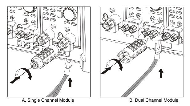
Figure 2-5 Load Connection with the Tailor-made Spanner
