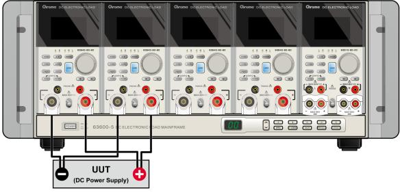
Figure 2-6 Parallel Connection
