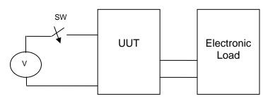
Figure 3-23 Power, UUT & Electronic Load Connecting Diagram
