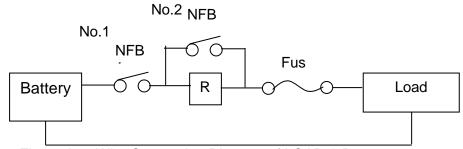
Figure A-3 Wire Connecting Diagram of LOAD & Battery **NFB(No-Fuse Breaker)**: The capacity (current amount) should be smaller than maximum current to facilitate load and it should be able to cutoff in time when the internal is aging short circuited.
